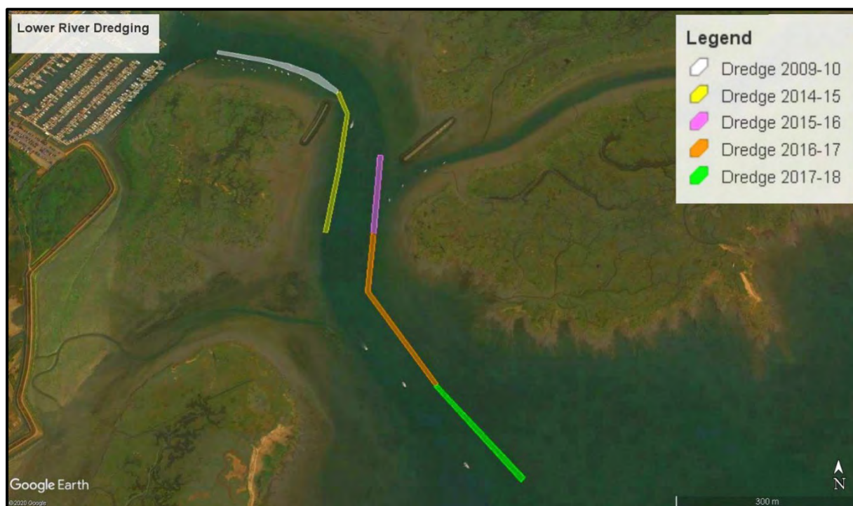
Image 1. Location and timing of LHC lower river capital dredging campaigns
