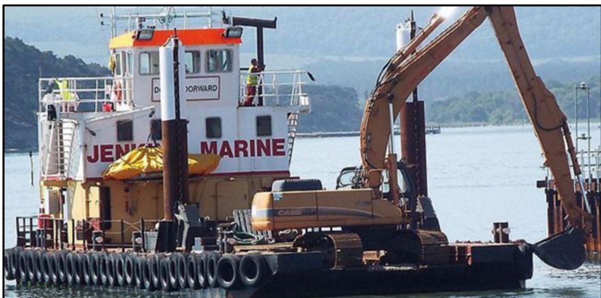
Image 3. Jenkins Marine's 'Doreen Dorward' self-propelled pontoon with excavator
